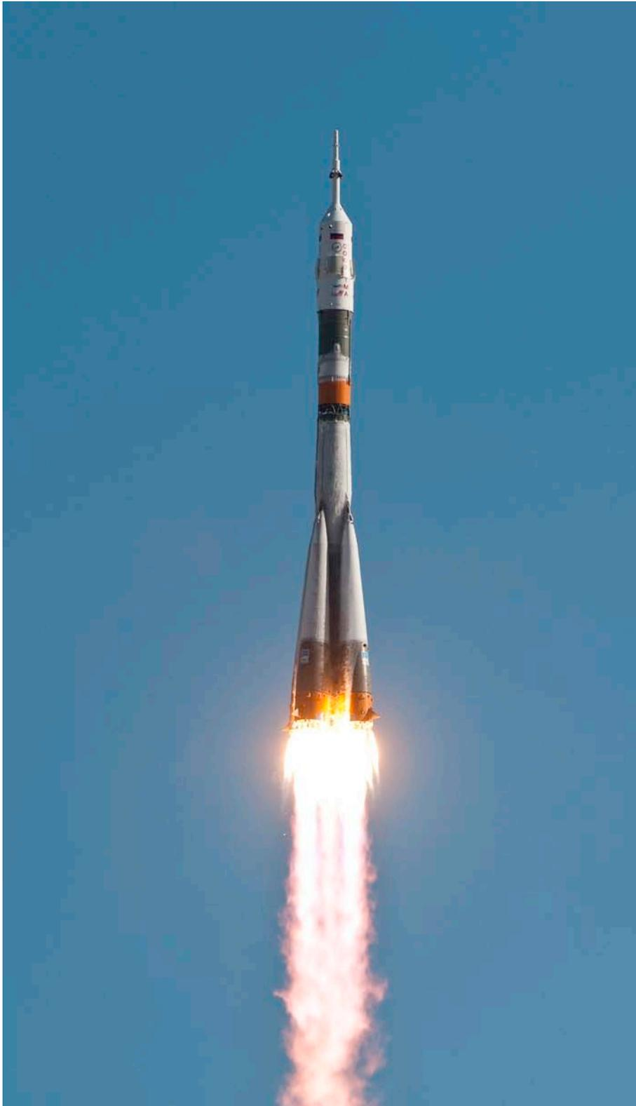
The sky's the limit! The highly concentrated hydrogen peroxide - 82.5 percent - drives the turbo pumps that force the actual fuels - kerosene and liquid oxygen - into the combustion chambers.
