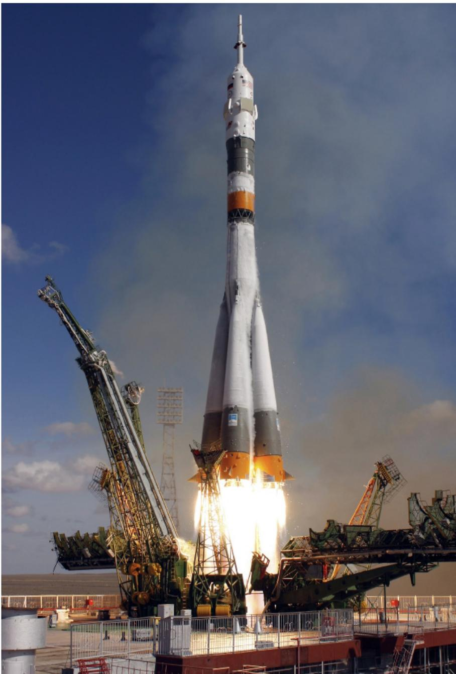
The sky's the limit! The highly concentrated hydrogen peroxide - 82.5 percent - drives the turbo pumps that force the actual fuels – kerosene and liquid oxygen – into the combustion chambers.
